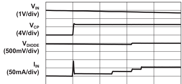
Load Switch to Charge Pump (1.5X Mode, 3x30mA Load)
